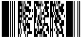
The PDF417 barcode encoded with the same data but with 2 columns is shown in the diagram below.
